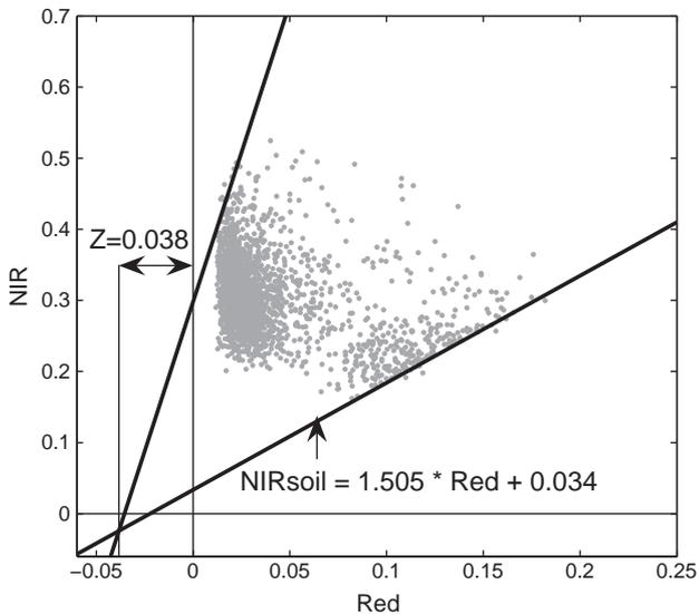
**Fig. 4.** NIR reflectance versus red reflectance for all stands listed in Table 1, for their entire rotation. This reflectance triangle was used to estimate the values of the GESAVI parameters. The soil line (corresponding to LAI=0) is shown, together with an estimation of the value of parameter  $Z$ .
